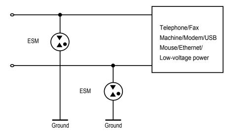
These ESM absorbers protect against common-mode interference voltages, i.e. surge voltages that appear in both exchange lines connecting to the ground. in the event of voltage overload, the ESM protects both exchange lines by conducting the surge current away to the ground.
